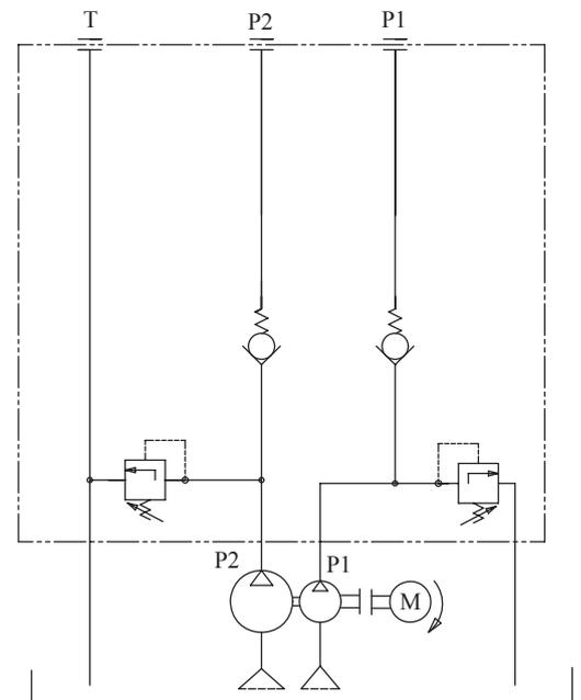
The W85AB series power pack is designed for applications that need two independent hydraulic power supply, but only use a single B14 Frame motor.
